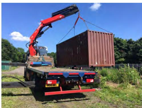
Loading the container on to the truck
